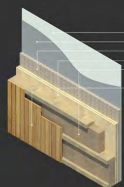
TRASMITTANZA  $U=0,184 \text{ W/m}^2\text{K}$  ✓
